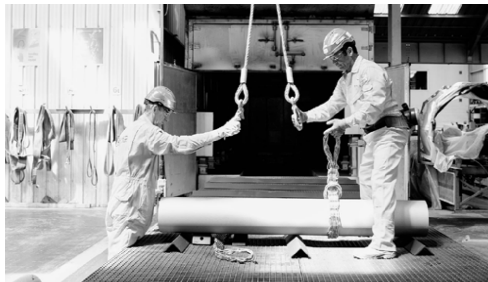
Heated pipe before application of epoxy powder
